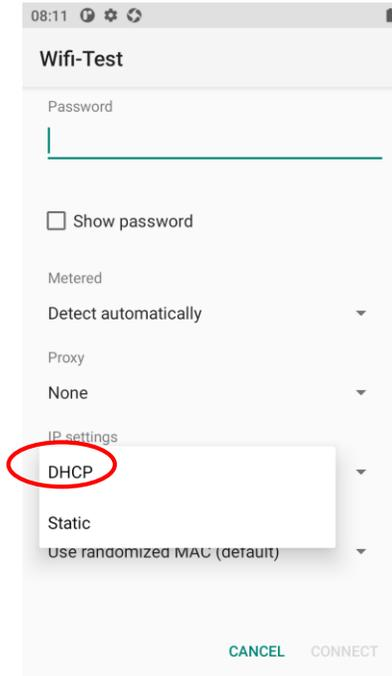
2. Select “Static” to customize the IP address. This will help to avoid the network failure caused by the duplication of the IP address in the LAN or the disable of the DHCP service in the router etc.
