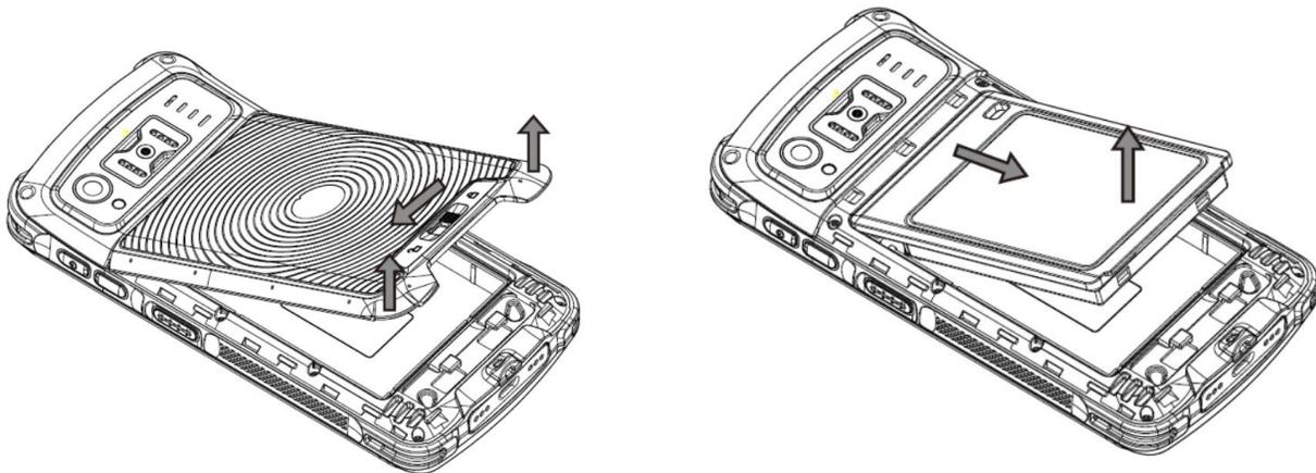
Step 1: Hold down the Power key for 5 seconds and then tap "Power off" to turn off the terminal. Slide the battery cover latch to the unlock position and remove the cover.
