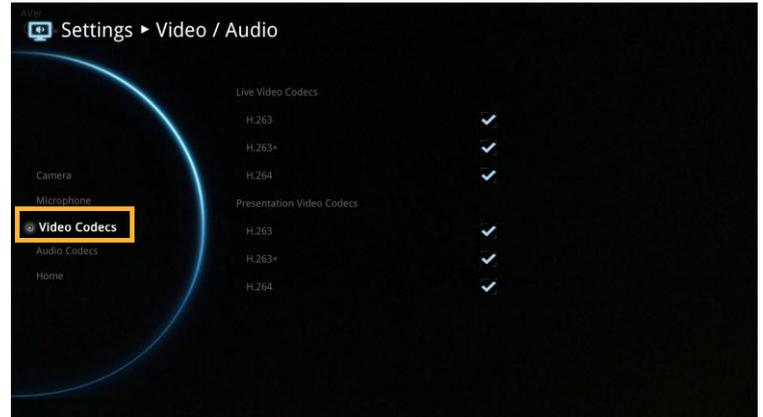
Select the **Video/Audio Codecs** to specify the codecs you want to support. While the Aver EVC supports the H.323 standard coding algorithm, each codec has unique properties and performs best given a certain set of circumstances.
